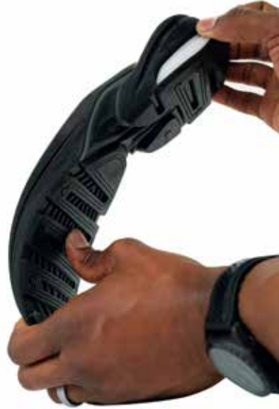
Shoe sole printed in a combination of flexible black elastomer and rigid white plastic
