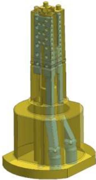
The image to the left shows the core in a translucent state so as to see the cooling channels. It is important to note that the primary channel is created by simply offsetting the core surfaces and then adding connector bosses for strength.
