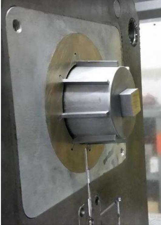
Bastech makes several versions of this core with a 3/8" NPT baffle running up the center. The most recent style brought the opportunity to manufacture the core with AM (maraging steel) and conformal cooling.
