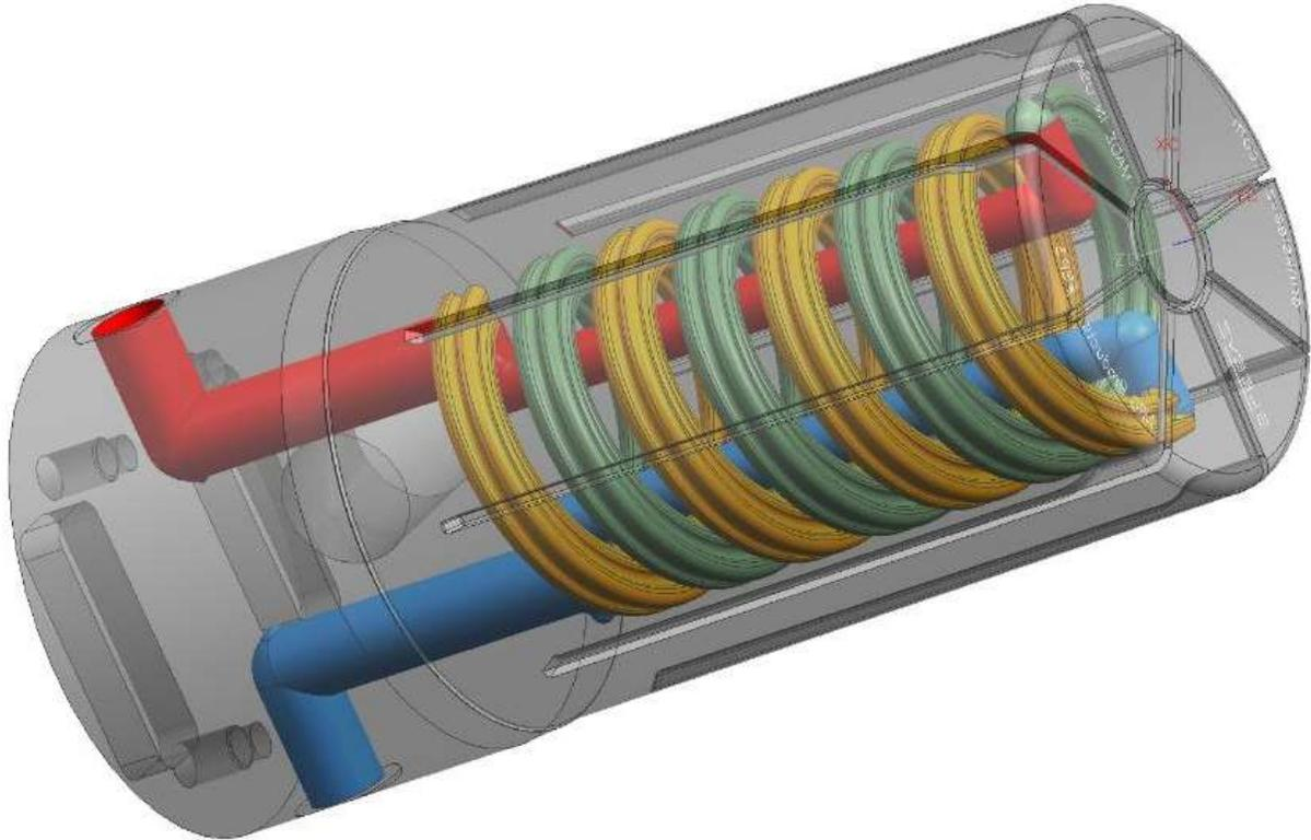
The image above is an example of a reverse flow helix. The supply side is shown in blue and splits into two helical channels. One (green) starts from the base and works to the end of the core while the other (yellow) starts at the end of the core and flows to the base of the insert. In this case, the channels were designed to precisely split the cross-sectional area of the supply (and return) in half to maintain flow without dead pockets.
