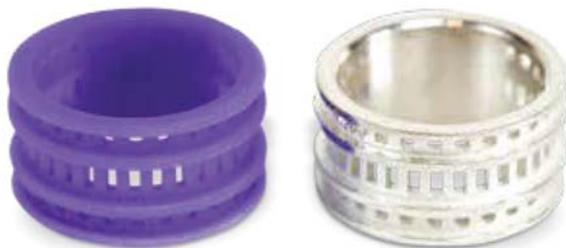
Ring printed in Visijet M2 CAST and cast
